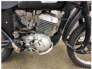
Terry found me some banana forks. I built a wide ratio gearbox with four evenly spaced ratios, 21" front wheel, trials tyres and a high level exhaust and I was on the way. I have to say that the initial rides were a disappointment, the Siba would only crank a low compression engine and not enough power. I replaced the iron cylinder with an Anglian top half and machined the head to take a Bond Minicar compression reducer so that I could
